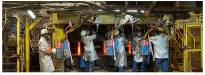
Continuous casting at Ugine melting shop
